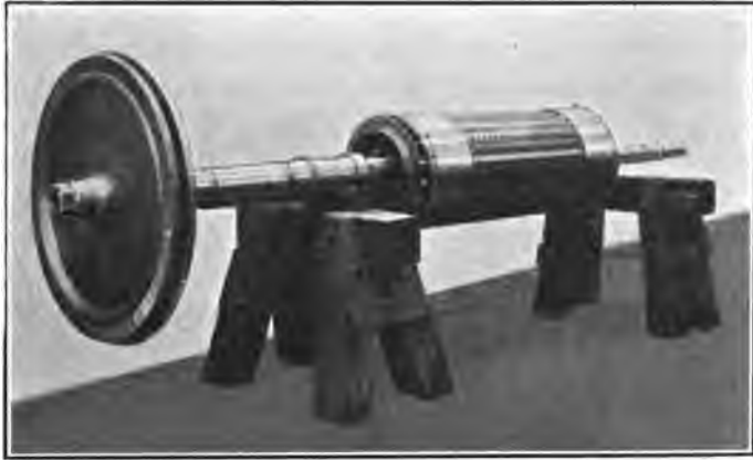
FIG. 68.—Rotor of 1000-H.P. machine.
